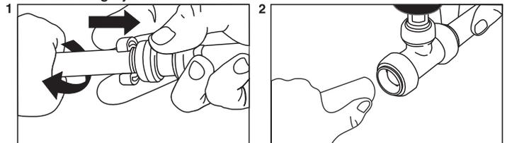
Push the disconnecting clip against the release collar and pull the pipe with a twisting action.
